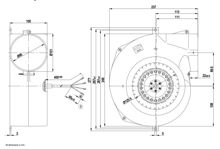
Cable PVC 4x 0.5 mm², 4x crimped splices
