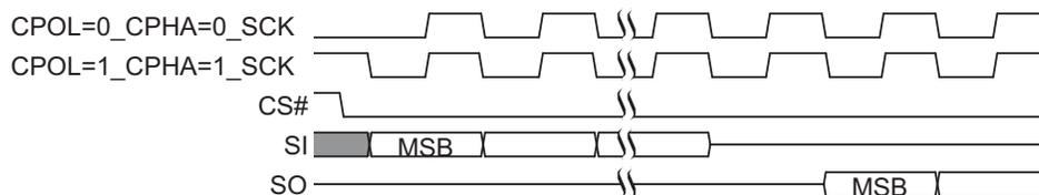
Timing diagrams throughout the remainder of the document are generally shown as both mode 0 and 3 by showing SCK as both high and low at the fall of CS#. In some cases a timing diagram may show only mode 0 with SCK low at the fall of CS#. In such a case, mode 3 timing simply means clock is high at the fall of CS# so no SCK rising edge set up or hold time to the falling edge of CS# is needed for mode 3.
