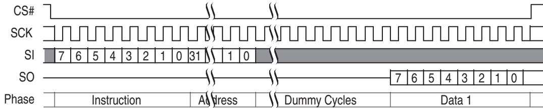
Figure 12. Dual Output Command
