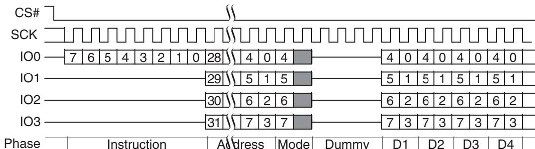
Figure 16. DDR Fast Read with EHPLC = 00b
