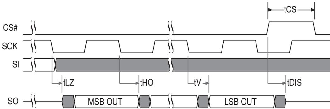
**Figure 33. SPI SDR MIO Timing**
