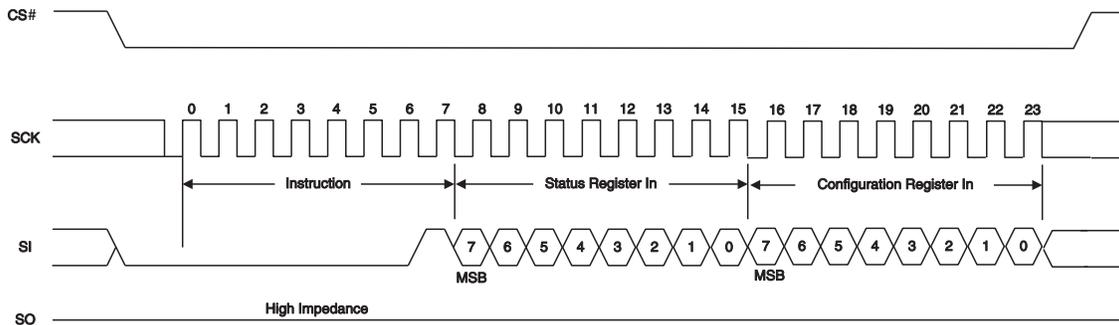
The Write Registers (WRR) command allows the user to change the values of the Block Protect (BP2, BP1, and BP0) bits to define the size of the area that is to be treated as read-only. The Write Registers (WRR) command also allows the user to set the Status Register Write Disable (SRWD) bit to a 1 or a 0. The Status Register Write Disable (SRWD) bit and Write Protect (WP#) signal allow the BP bits to be hardware protected.
