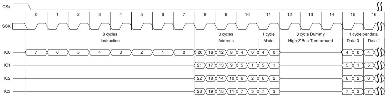
**Figure 9.31** Continuous DDR Quad I/O Read Subsequent Access (3-byte Address, HPLC=11b)
