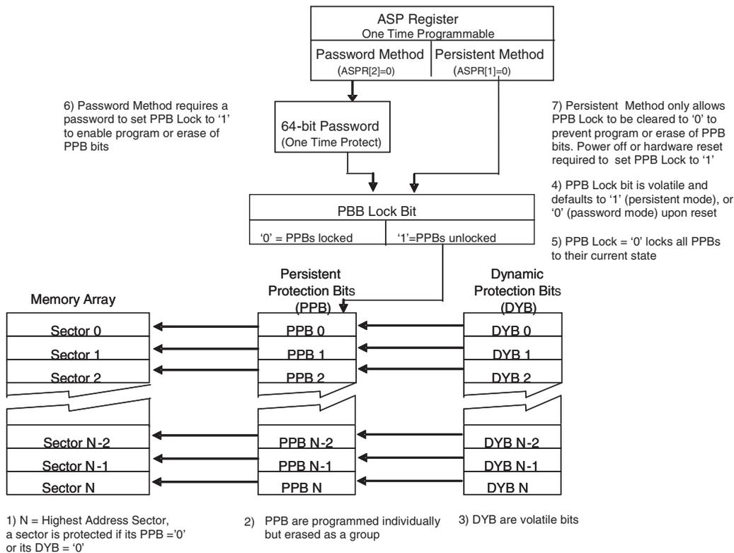
Every main flash array sector has a non-volatile (PPB) and a volatile (DYB) protection bit associated with it. When either bit is 0, the sector is protected from program and erase operations.
