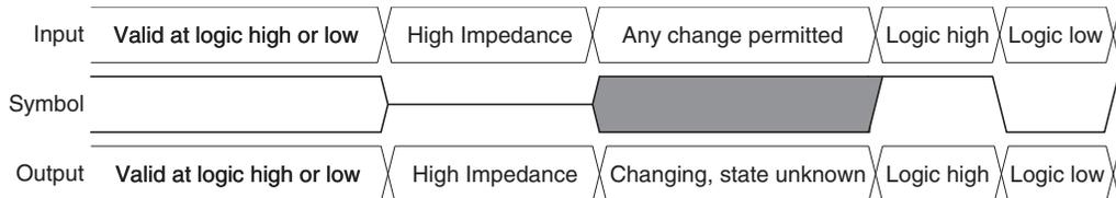
Figure 24. Input, Output, and Timing Reference Levels
