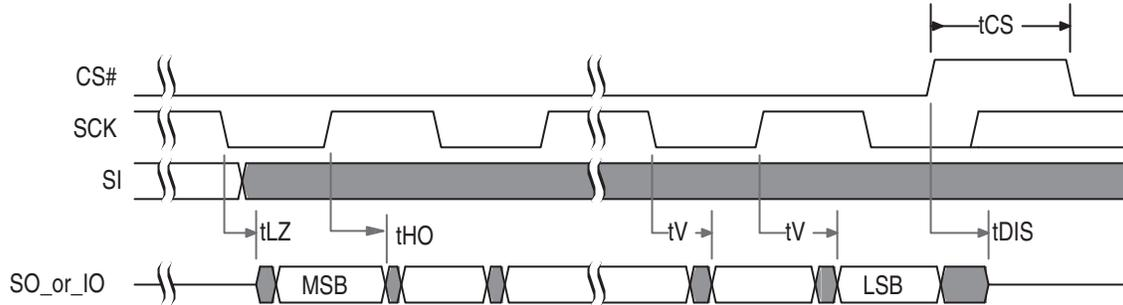
Figure 37. SPI DDR Data Valid Window
