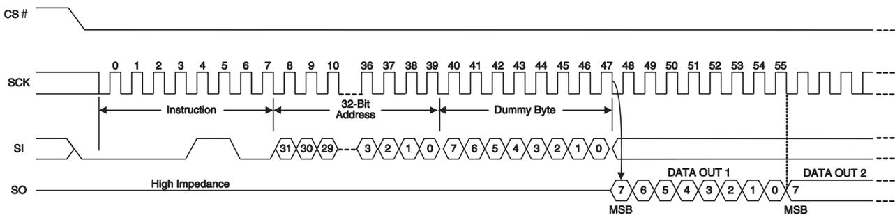
**Figure 9.10** Fast Read Command Sequence (4-byte Address, 0Ch or 0B [ExtAdd=1], LC=11b)
