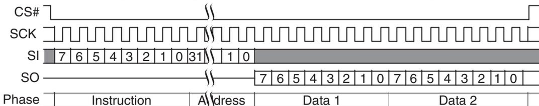
Figure 11. Single Bit Wide I/O Command with Latency
