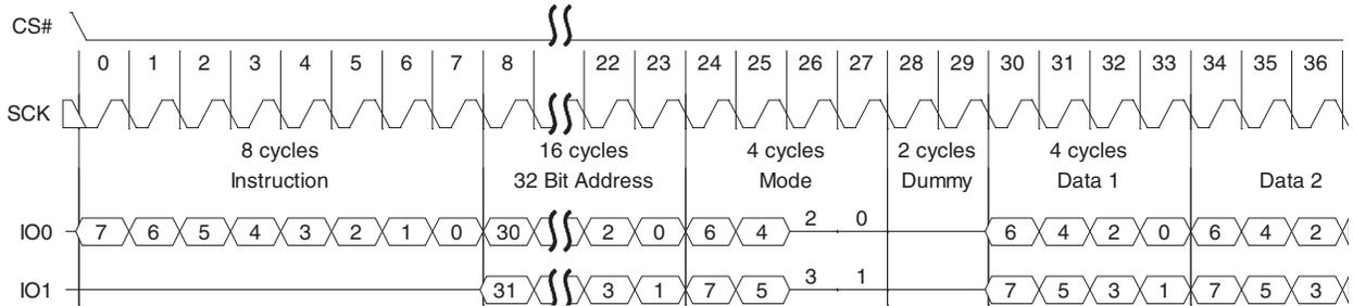
**Figure 63. Continuous Dual I/O Read Command Sequence (4-byte Address, BCh or BBh [ExtAdd=1], EHPLC=10b)**
