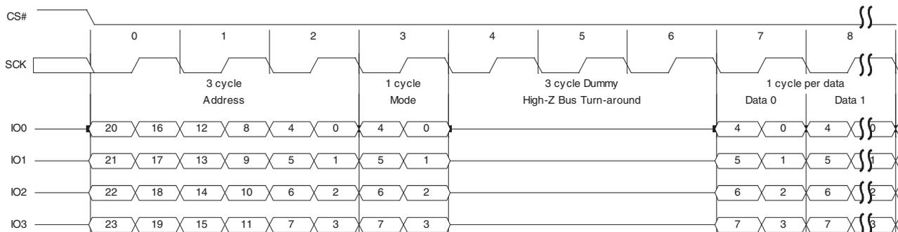
**Figure 9.32** DDR Quad I/O Read Initial Access (4-byte Address, EEh or EDh [ExtAdd=1], EHPLC=01b)
