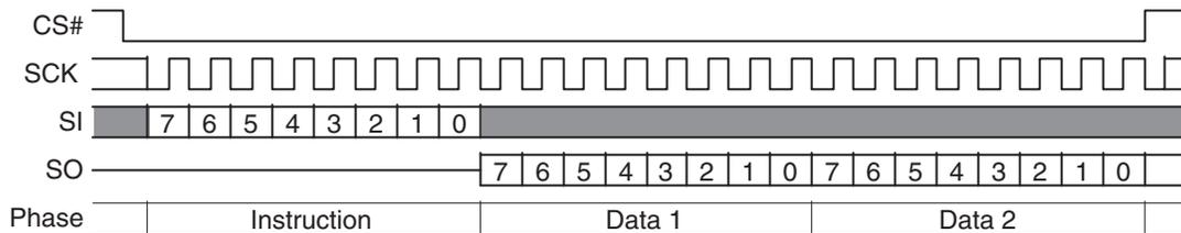
**Figure 10. Single Bit Wide I/O Command without Latency**
