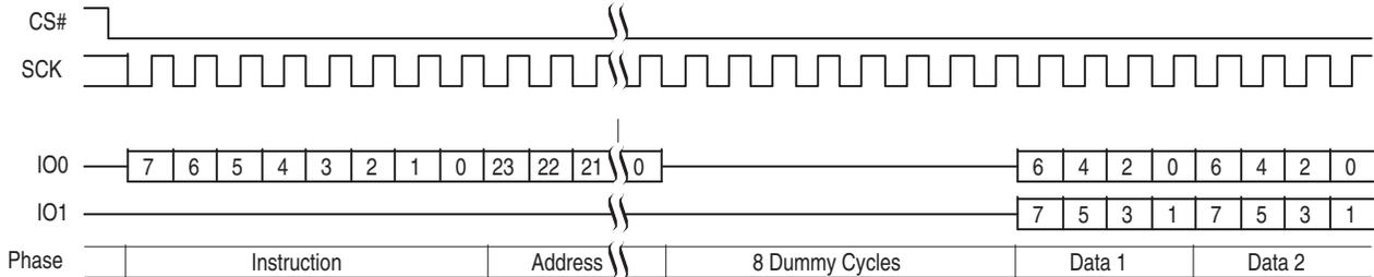
**Figure 9.12** Dual Output Read Command Sequence (4-byte Address, 3Ch or 3Bh [ExtAdd=1, LC=10b])
