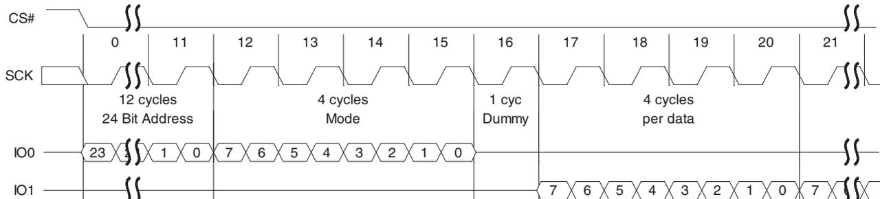
**Figure 9.24** DDR Fast Read Initial Access (4-byte Address, 0Eh or 0Dh [ExtAdd=1], EHPLC=01b)
