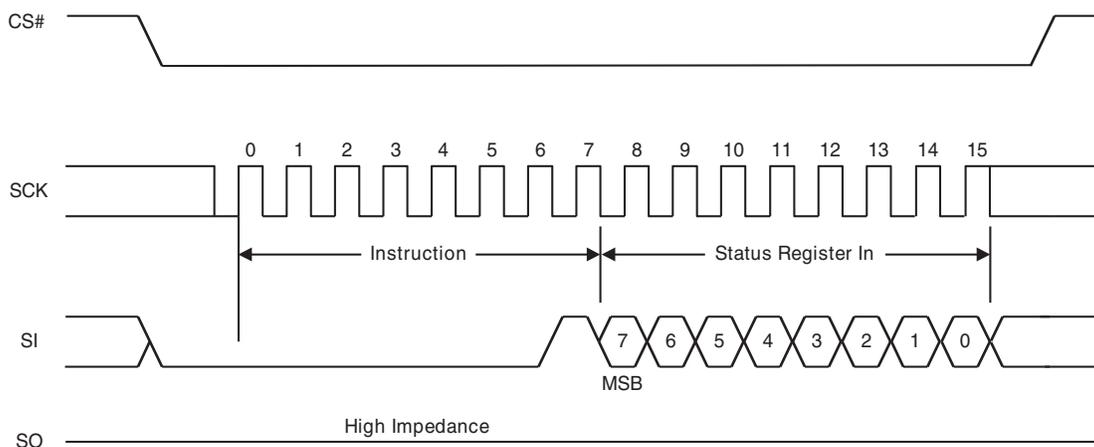
Figure 50. Write Registers (WRR) Command Sequence – 16 data bits
