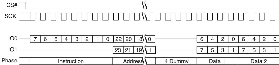
**Figure 9.16 Dual I/O Read Command Sequence (4-byte Address, BBh [ExtAdd=1], HPLC=10b)**
