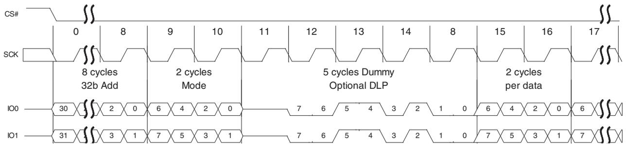
**Figure 9.29** DDR Dual I/O Read (4-byte Address, BEh or BDh [ExtAdd=1], HPLC=00b)
