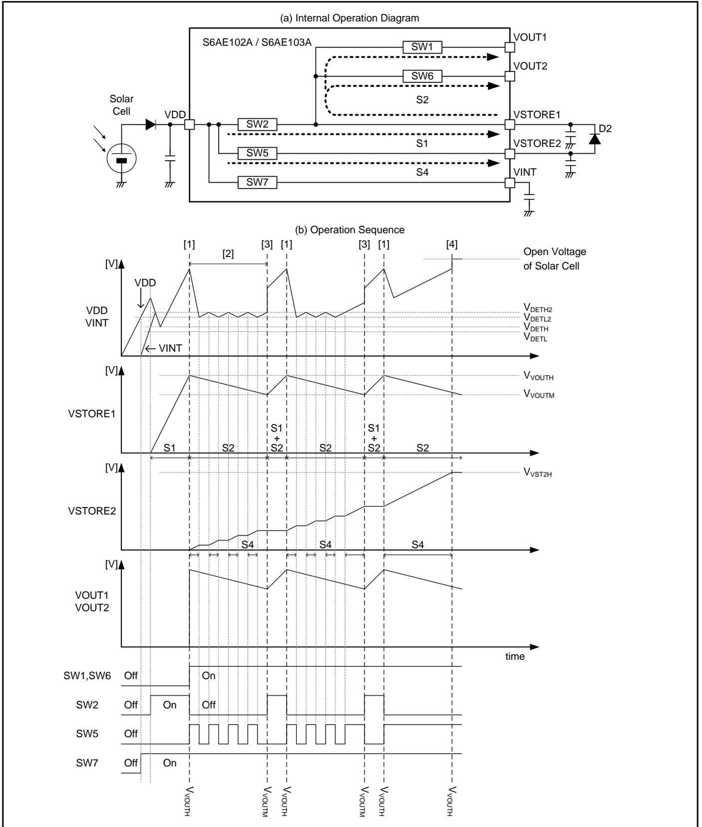
**VSTORE2 Input Power Operation ( $V_{\text{SYSH}} \geq 2.5\text{V}$ )**
