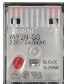
Relay with AC Coil (LED: Red)
