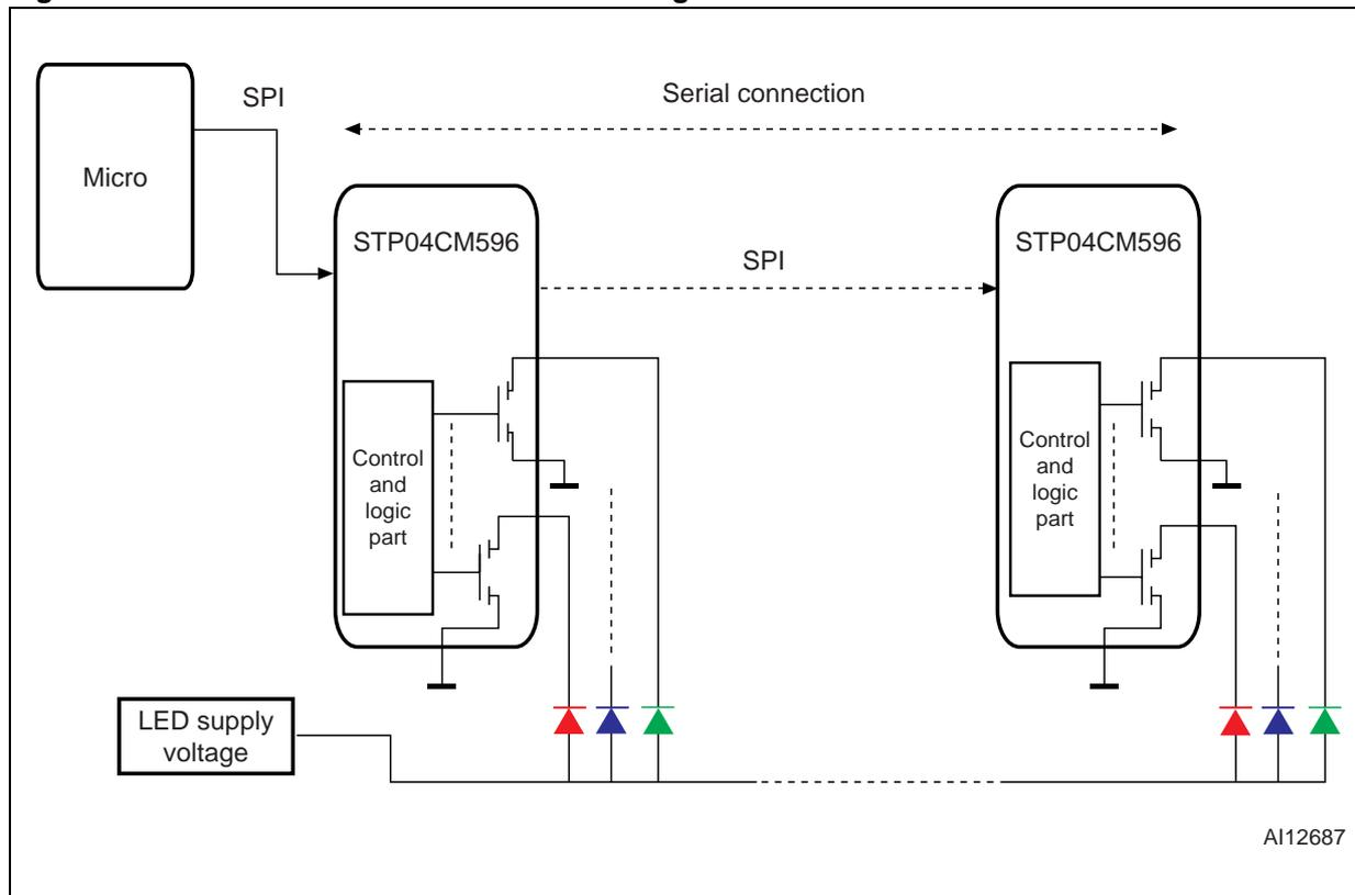
Figure 4. LED driver connection - parallel configuration
