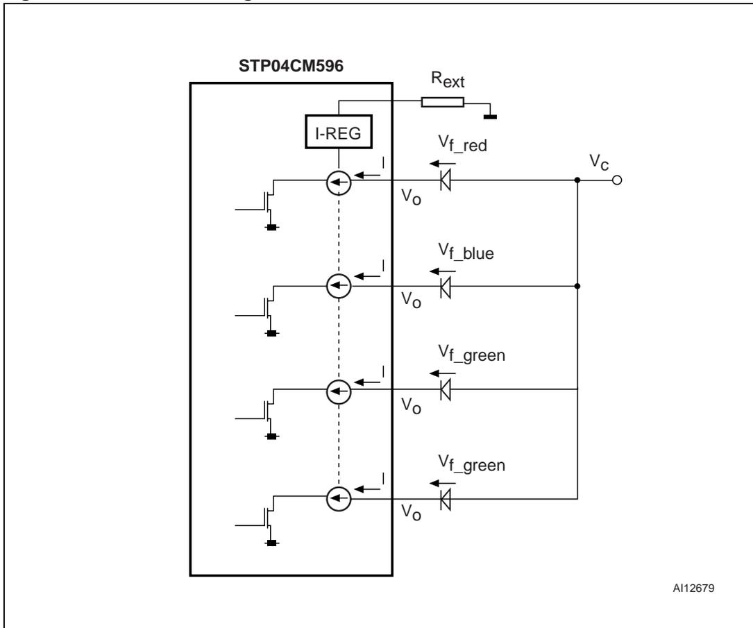
*Note:* Red, blue and green LEDs have different forward voltages (refer to [Chapter 2](#)). In general, the red LED has a lower forward voltage and therefore the power dissipation on the red LED channel is the highest. There is quite simple way to decrease this power dissipation by using a serial resistor with the red LED. Calculation example is shown in [Section 9.1](#) and [10.1](#).
