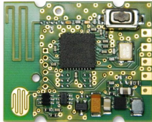
ECO 200 or ECO 250 can be either mechanically connected using two contact pairs or wired to the electrical interface of PTM 535Z.
