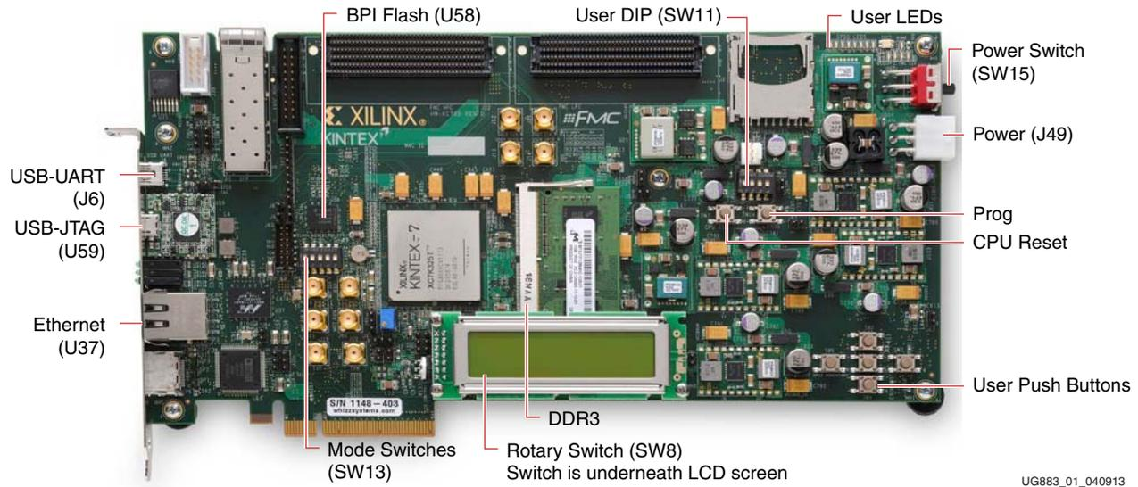
Figure 1: KC705 Board Features Used by the BIST
