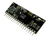
**BRAVO-T433** - 433MHz SMART Radio Module with 8 digital outputs. **BRAVO-T868** - 868 MHz SMART Radio Module with 8 digital outputs.
