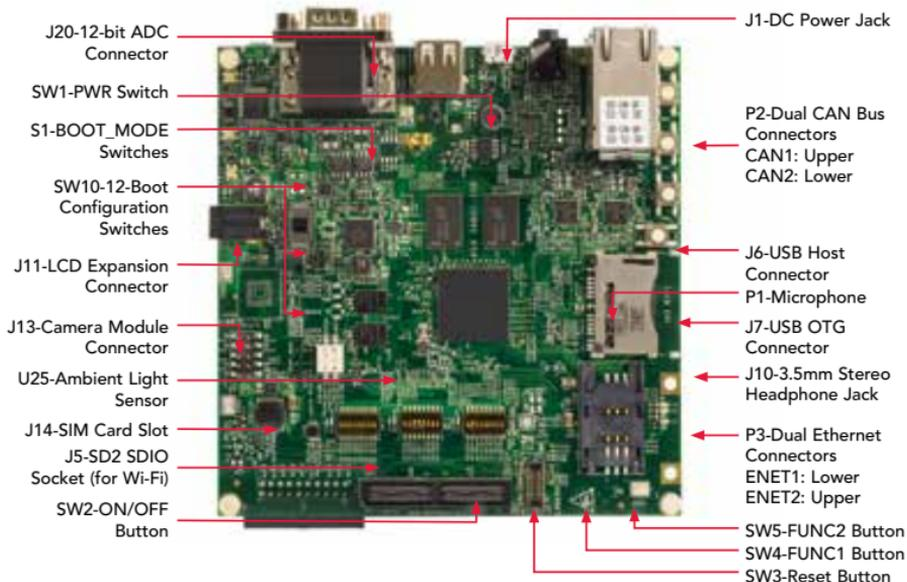
Figure 1: Front side of i.MX 6SoloX SABRE-SDB (top)
