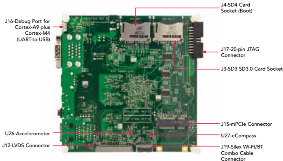
Figure 2: Back side of i.MX 6SoloX SABRE-SDB (bottom)
