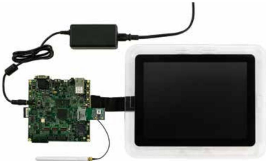
Example system set up with SABRE Board for Smart Devices based on i.MX 6SoloX
