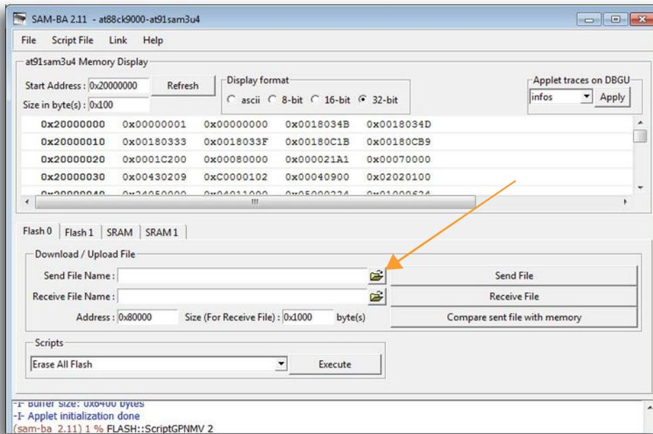
14. Find the binary firmware file located in the directory, **at88ck9000\_fw**. The name of the firmware file could change based on the version.
