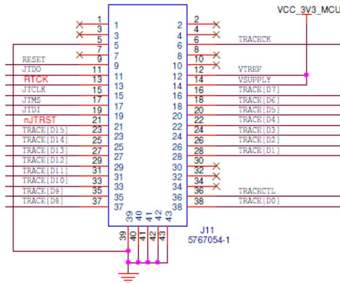
Figure 10. 38-pin Mictor connector
