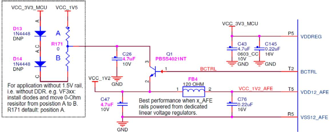
Figure 8. Hybrid core power
