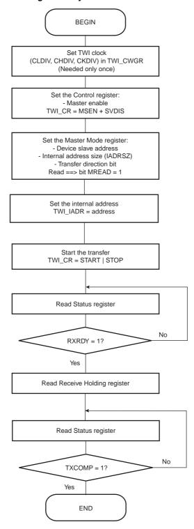
Figure 30-19. TWI Read Operation with Multiple Data Bytes with or without Internal Address
