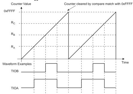
Figure 33-8. WAVSEL = 00 with trigger
