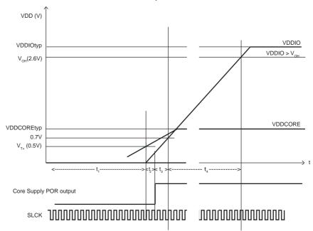
Figure 4-1. VDDCORE and VDDIO Constraints at Startup
