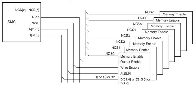
Figure 20-2. Memory Connections for Eight External Devices
