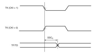
Figure 40-14. SSC Transmitter, TK in Input and TF in Output
