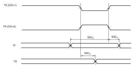
Figure 40-16. SSC Transmitter, TK and TF in Input
