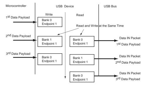
When using a ping-pong endpoint, the following procedures are required to perform Data IN transactions:
