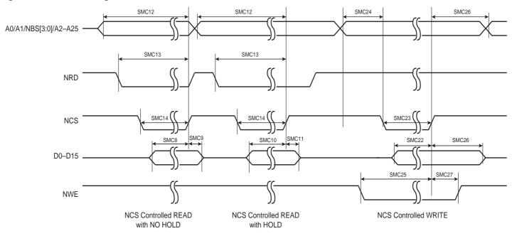
Figure 40-5. SMC Timings - NRD Controlled Read and NWE Controlled Write
