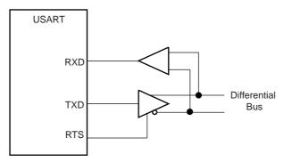
The USART is set in RS485 mode by programming the USART\_MODE field in the Mode Register (US\_MR) to the value 0x1.
