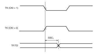
Figure 40-15. SSC Transmitter, TK in Output and TF in Input
