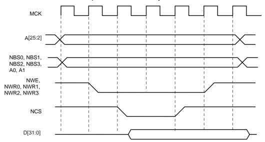
Figure 20-15. WRITE\_MODE = 0. The write operation is controlled by NCS
