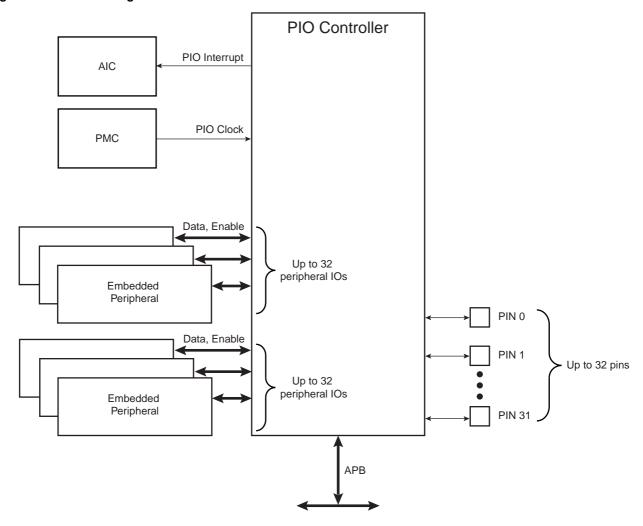
Figure 28-2. Application Block Diagram
