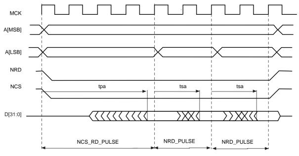
The NRD and NCS signals are held low during all read transfers, whatever the programmed values of the setup and hold timings in the User Interface may be. Moreover, the NRD and NCS timings are identical. The pulse length of the first access to the page is defined with the NCS\_RD\_PULSE field of the SMC\_PULSE register. The pulse length of subsequent accesses within the page are defined using the NRD\_PULSE parameter.
