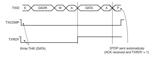
Figure 30-7. Master Write with Multiple Data Byte
