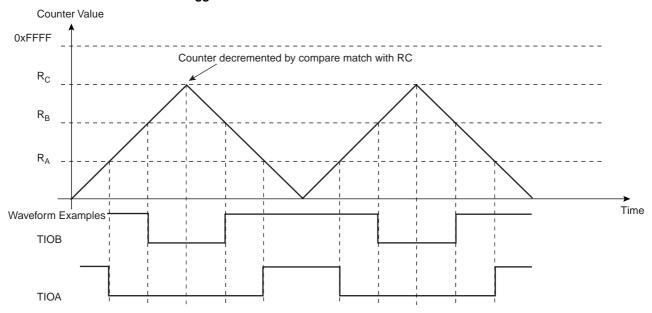
Figure 33-14. WAVSEL = 11 With Trigger
