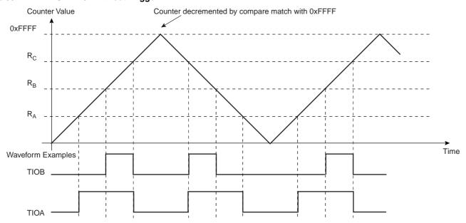
Figure 33-12. WAVSEL = 01 With Trigger
