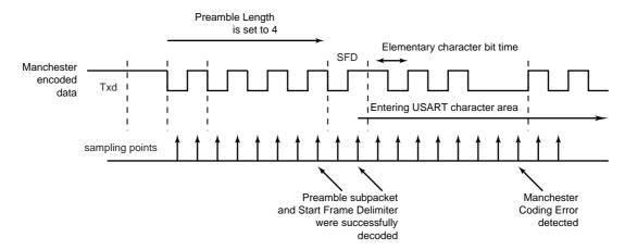
When the start frame delimiter is a sync pattern (ONEBIT field at 0), both command and data delimiter are supported. If a valid sync is detected, the received character is written as RXCHR field in the US\_RHR and the RXSYNH is updated. RXCHR is set to 1 when the received character is a command, and it is set to 0 if the received character is a data. This mechanism alleviates and simplifies the direct memory access as the character contains its own sync field in the same register.
