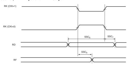
Figure 40-19. SSC Receiver, RK and RF in Output
