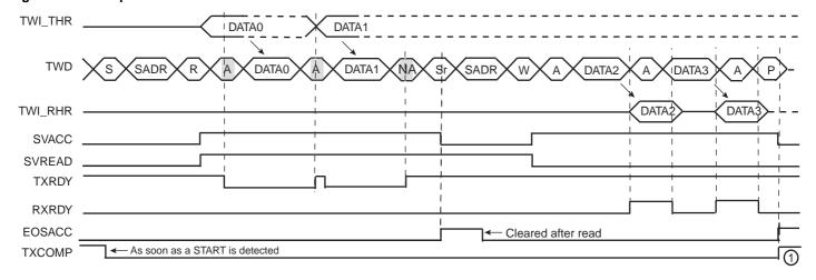
Note: 1. TXCOMP is only set at the end of the transmission because after the repeated start, SADR is detected again.
