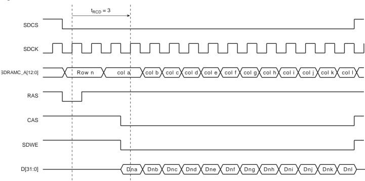
Figure 21-2. Write Burst, 32-bit SDRAM Access
