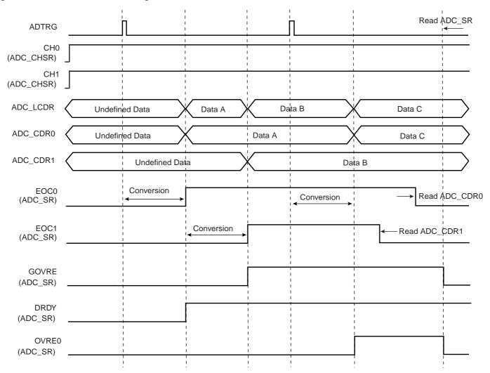
**Warning:** If the corresponding channel is disabled during a conversion or if it is disabled and then reenabled during a conversion, its associated data and its corresponding EOC and OVRE flags in ADC\_SR are unpredictable.
