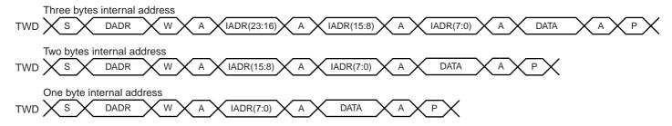
Figure 30-12. Master Read with One, Two or Three Bytes Internal Address and One Data Byte
