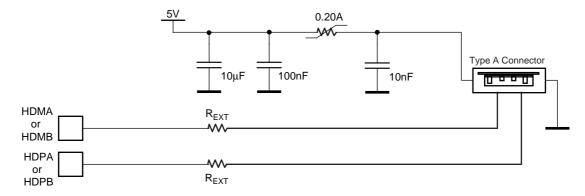
A termination serial resistor must be connected to HDP and HDM. The resistor value is defined in the electrical specification of the product  $(R_{EXT})$ .
