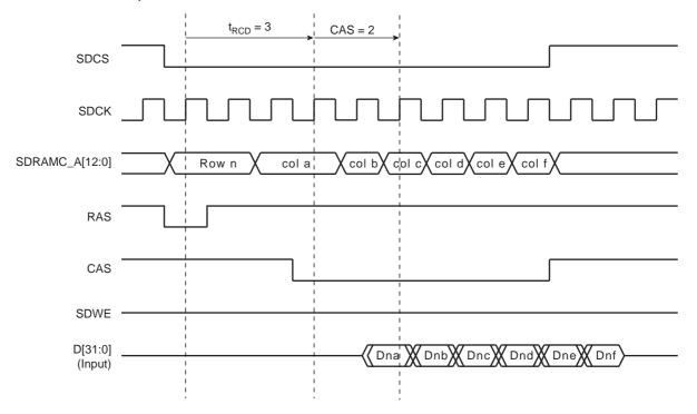
Figure 21-3. Read Burst, 32-bit SDRAM Access
