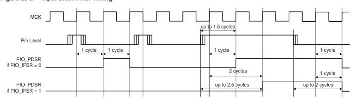
Figure 28-5. Input Glitch Filter Timing
