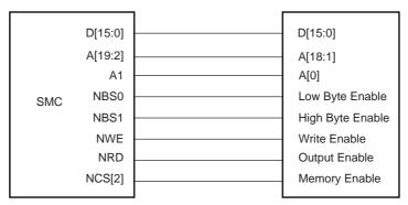
Figure 20-5. Memory Connection for a 32-bit Data Bus
