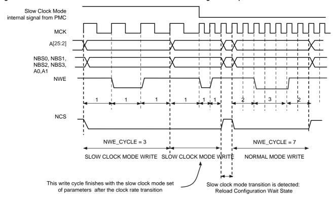
Figure 20-33. Recommended Procedure to Switch from Slow Clock Mode to Normal Mode or from Normal Mode to Slow Clock Mode
