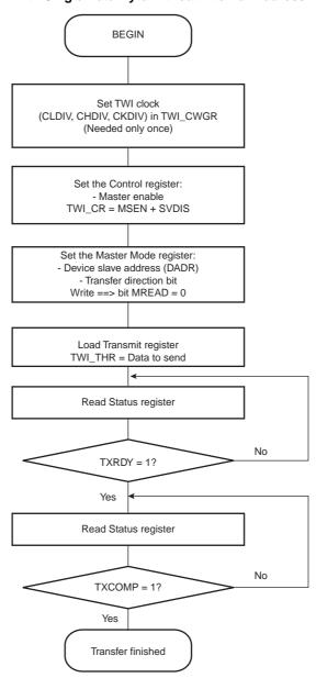
Figure 30-15. TWI Write Operation with Single Data Byte and Internal Address
