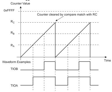
Figure 33-10. WAVSEL = 10 With Trigger
