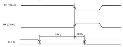
Figure 40-18. SSC Receiver, RK in input and RF in Output
