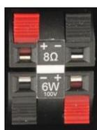
When used with a standard (non-100V) amplifier, connect to the "8Ω" terminals and refer to the amplifier manufacturer's manual to ensure that total speaker impedance ( $\Omega$ ) is not less than recommended for the amplifier.
