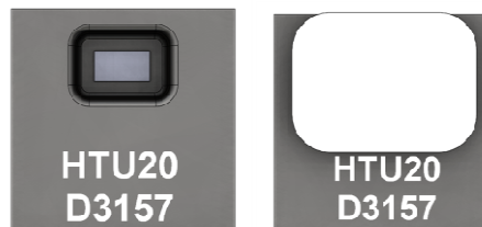
Laser marking on HTU20D(F) sensor
