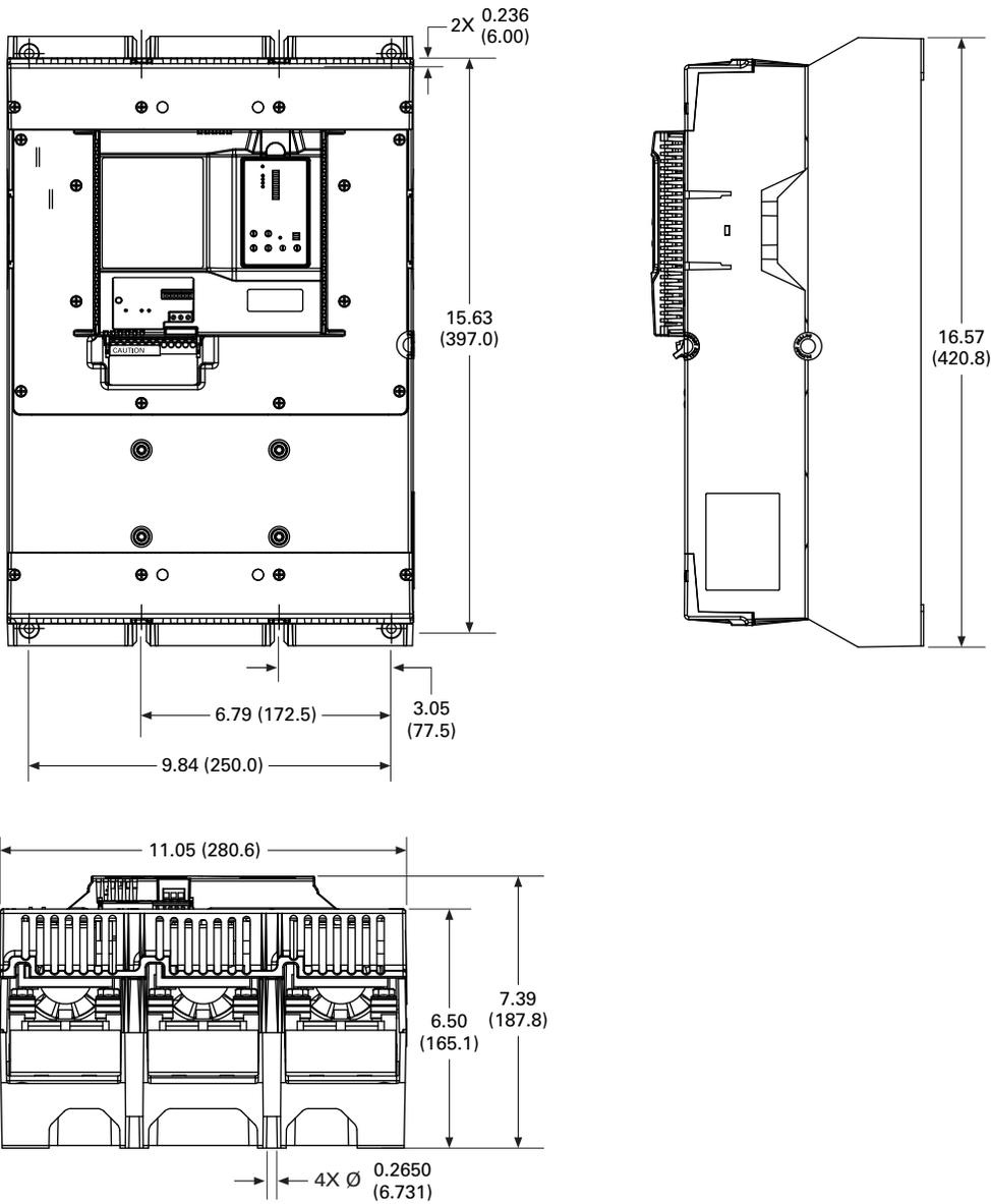
Type S811+, Soft Starters with Digital Interface Module (DIM)
