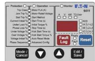
The UI can be removed from the S611 and remote mounted. Kits are available to door mount the UI, enabling users to safely configure, commission, monitor and troubleshoot the system at the electrical panel without opening the enclosure door. This will help eliminate the possibility of an arc flash incident.
