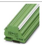
Input solid-state relay terminal block, input: 5 V DC, output: 3 - 48 V DC/100 mA, terminal block width: 6.2 mm
