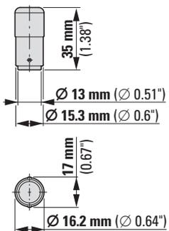
Tool for replacing filament lamp
