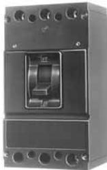
**Type DA Breakers 250–400A, 240 Vac, 250 Vdc, Two- and Three-Pole, Fixed Trip, Thermal-Magnetic (Suitable for Reverse-Feed)**
