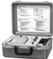
Provides verification of performance of all frame sizes of SELTRONIC breakers while devices are still in service under varying load and/or phase unbalance. The tester operates on 120V, 50/60 Hz, and includes complete instructions and test times for testing the long time, instantaneous operation and optional ground fault operation of the breaker.
