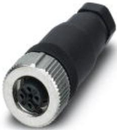
Sensor/actuator connector, female, straight, 5-pos., M12 SPEEDCON, A-coded, screw connection, metal knurl, cable screw connection Pg7
