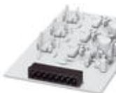
Header, Nominal current: 12 A, Rated voltage (III/2): 320 V, Number of positions: 3, Pitch: 5.08 mm, Color: black, Contact surface: Tin, Mounting: THR soldering, User information and design recommendations for through hole reflow technology can be found under "Downloads"
