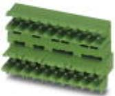
Header, Nominal current: 10 A, Rated voltage (III/2): 320 V, Number of positions: 3, Pitch: 5.08 mm, Color: green, Contact surface: Tin, Mounting: Wave soldering, The article can be aligned to create different nos. of positions! In combination with MVSTB or FKCV plug components, both an MVSTBW (or FKCVW) and an MVSTBR plug (or FKCVR) must be used. Combination with TMSTBP plug components is not possible!
