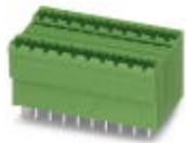
Header, Nominal current: 10 A, Rated voltage (III/2): 320 V, Number of positions: 3, Pitch: 5.08 mm, Color: green, Contact surface: Tin, Mounting: Wave soldering, In combination with MVSTB or FKCV plug components, both an MVSTBW (or FKCVW) and an MVSTBR plug (or FKCVR) must be used. Combination with TMSTBP plug components is not possible!
