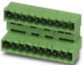
Header, Nominal current: 10 A, Rated voltage (III/2): 320 V, Number of positions: 3, Pitch: 5.08 mm, Color: green, Contact surface: Tin, Mounting: Wave soldering, The article can be aligned to create different nos. of positions! In combination with MVSTB or FKCV plug components, both an MVSTBW (or FKCVW) and an MVSTBR plug (or FKCVR) must be used. Combination with TMSTBP plug components is not possible!
