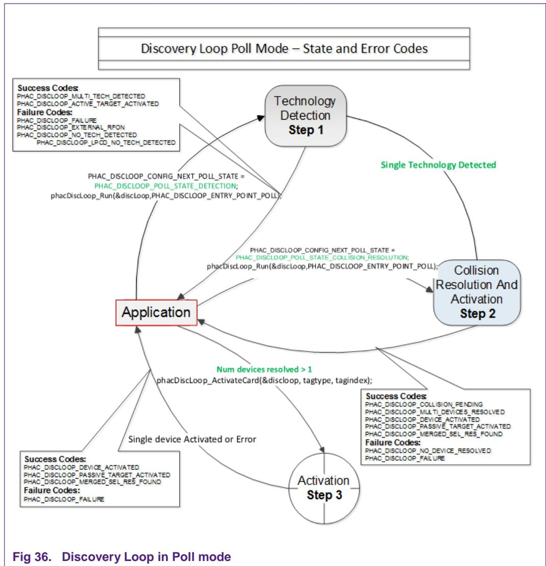
The core function of this example is “*BasicDiscoveryLoop\_Demo()*”, where initialization of the NFC Reader library and polling for NFC technologies is implemented. After each polling loop, application is checking polling result and printout information about the detected tags or devices.
