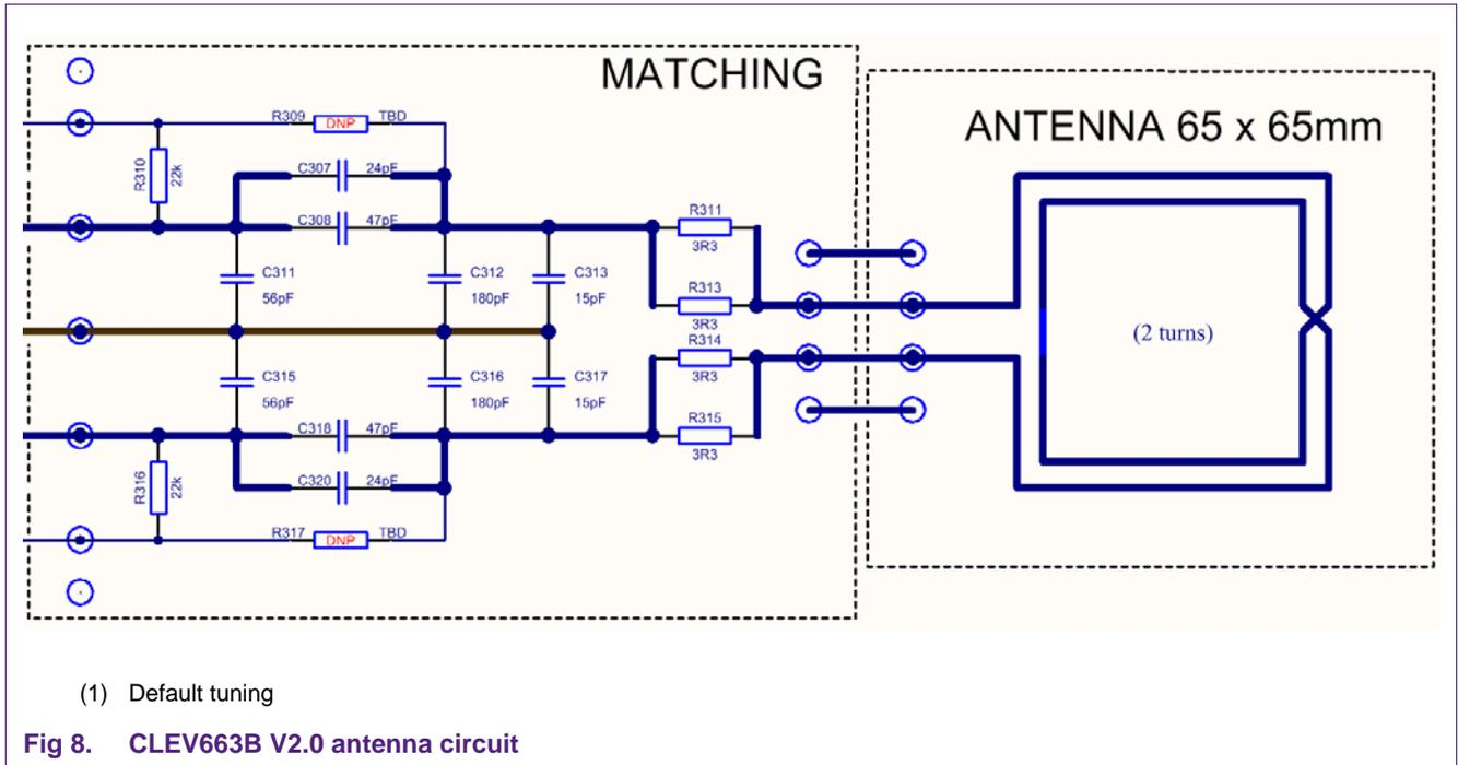
The “asymmetrical” tuning (see Fig 9) is a compromise to provide optimum power transfer and good wave shapes in combination with good loading effects, which automatically reduce the field strength under strong loading conditions.
