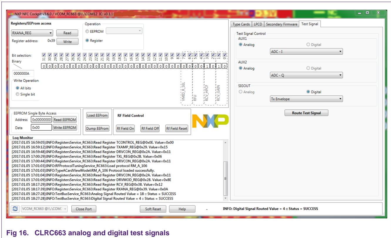
Fig 16. CLRC663 analog and digital test signals
