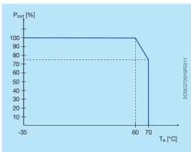
Characteristic curve of temperature at rated load
