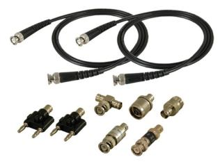
Model CC510 General Purpose Function Generator and Oscilloscope Kit provides a range of BNC and N Type coaxial interconnection for basic function / arbitrary waveform generators use. All components feature standard BNC or N Type interfaces with 50 ohm impedance and gold plated center contacts to ensure accurate repeatable measurements. The kit is provided in a convenient foam lined storage case for easy selection and use.
