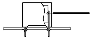
Temperature monitored inside the capacitor.
