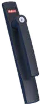
The L Handle is a stylish option for any solid, window or disconnect door, except Voice/Data or Colocation cabinets. It can be installed to rotate either clockwise or counterclockwise. Handle comes with a bezel, includes keylocking provision and is finished with RAL 9005 textured black polyester powder paint. Two keys are included. The bezel permits your logo to be inserted.
