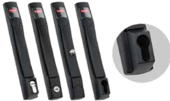
Flush Handles are optional for any solid, window or disconnect door greater than 600mm in height, except Voice/Data and Colocation cabinets. They are ergonomically designed to provide style and function in a low profile. The handle is die-cast zinc finished with RAL 9005 textured black polyester powder paint. Provision to add your logo is included. Handle can be installed to rotate either clockwise or counterclockwise.
