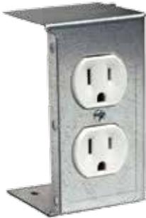
15 A duplex outlet is factory-mounted in three-sided, plated steel enclosure. Outlet enclosure mounts on hinge side of door in lower corner of cabinet. Mounting hardware provided.
