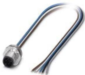
Sensor/actuator flush-type plug, 5-pos., M12-SPEEDCON, A-coded, front/screw mounting with M16 thread, with 0.5 m TPE litz wire, 5 x 0.34 mm<sup>2</sup>
