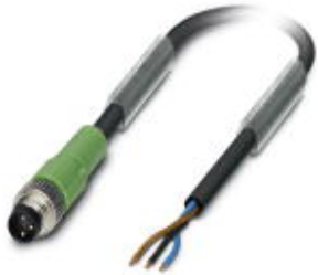
Sensor/Actuator cable, 3-position, PUR halogen-free, black-gray RAL 7021, Plug straight M8, on free cable end, Cable length: 10 m
