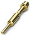
Crimp contact, turned, Single contact, Contact diameter: 1 mm, Crimp range: 0.34 mm<sup>2</sup>...0.5 mm<sup>2</sup>
