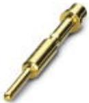
Crimp contact, turned, Single contact, Contact diameter: 1 mm, Crimp range: 0.5 mm<sup>2</sup>...1 mm<sup>2</sup>
