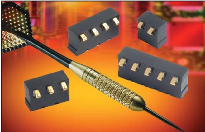
A further addition to the battery connector range offered by AVX is a 90 degree version. On a 3mm pitch, offered in 2 to 6 contact positions and rated as with all of the battery range at 3 amps. The connector's design is small and compact to minimize its profile yet stable while having a contact point 4.61mm above the PCB.
