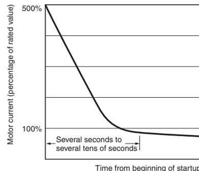
For a motor with a rating of 5 A, the startup current will be approximately 30 A. The startup current will exceed the overload capacity (rating: 150% for 1 s) of the K8DT-AS1 and K8DT-AS2 and result in failure of the Relay. To monitor the motor load, use the K8DT-AS3. (Overload capacity: 120% of rating for continuous load, 200% of rating for 30 s, and 600% of rating for 1 s). The K8DT-AS3 has a large input range. Pass the conductors multiple times through the special CT.
