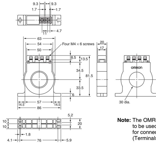
**Note:** The OMRON Current Transformer (CT) is designed to be used with the K8DT-AS3. Use terminals k and l for connections. (Terminals kt and lt are not used.)
