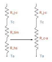
As the figure at right shows, the R\_c-a value is the sum of the thermal resistance of the TIM (R\_tim) plus the thermal resistance of the heat sink (R\_hs).
