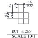
The non-specified tolerance of dimension is  $\pm 0.3 \text{ mm}$ .
