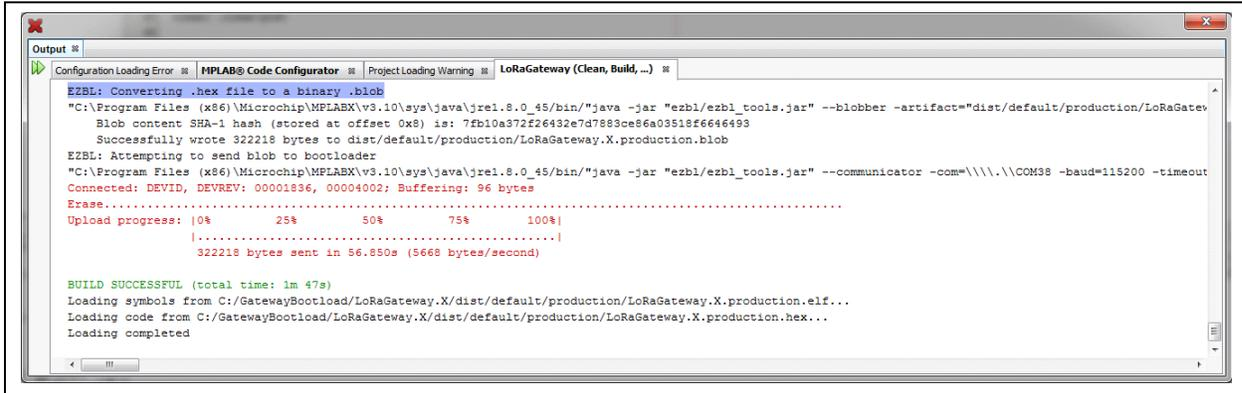
7. After the application code has been flashed, the Gateway board will automatically restart and the process is complete.
