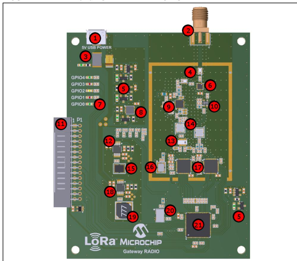
The LoRa Gateway Radio board captures all LoRa uplink packets using the two on-board SX1257 Semtech transceivers, and concentrates them into the SX1301 Base Band Processor. The 5V micro-USB B connector can be used to supply power to the
