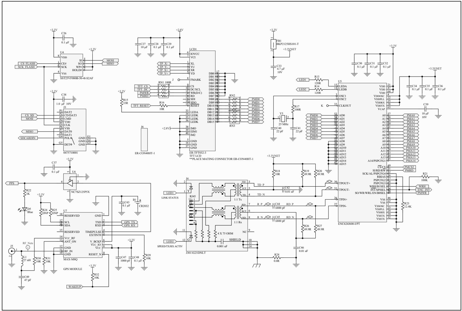
**FIGURE A-3: LoRa® GATEWAY CORE BOARD SCHEMATIC 3**
