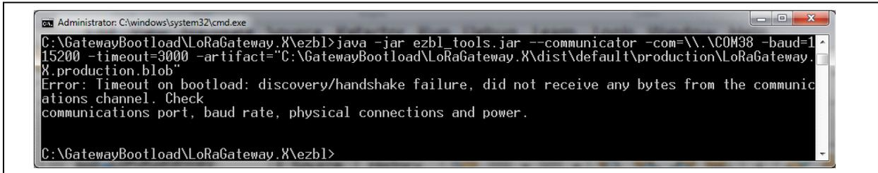
**Note:** If the bootloader fails to establish communication with the Gateway board, or if the time-out overlaps prior to pressing the **Reset** button, the command console will indicate the failure condition.
