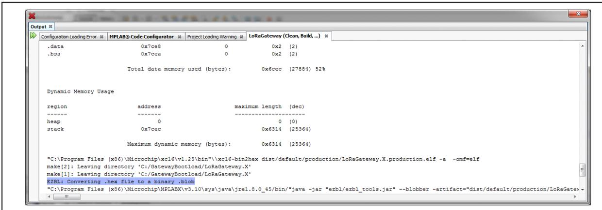
5. After the 2<sup>nd</sup> Echo message, the board is ready for the `.blob` file to be passed within the time-out period. The Output console will indicate progress.
