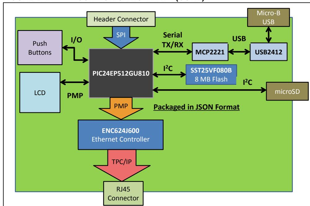
The LoRa Gateway Core board is populated with a PIC24EP512GU810 Microchip microcontroller. The MCU is responsible for capturing information passed by the LoRa Gateway Radio board, and forwarding the packet information to the Ethernet controller. The Radio board captures LoRa signals passively, concentrates the information, and passes data upon a fetch request by the connected board.
