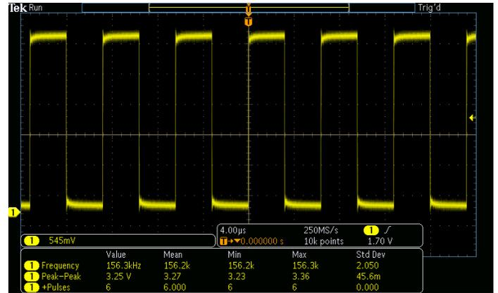
Automated measurement readouts provide repeatable, statistical views of waveform characteristics.
