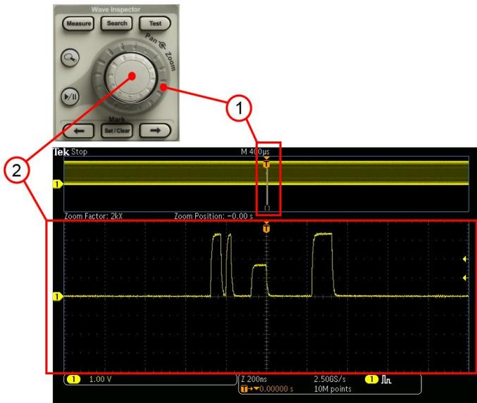
Wave Inspector controls provide unprecedented efficiency in viewing, navigating, and analyzing waveform data. Zip through your long record by turning the outer pan control (1). Get details from the beginning to end in seconds. See something of interest and want to see more details? Just turn the inner zoom control (2).
