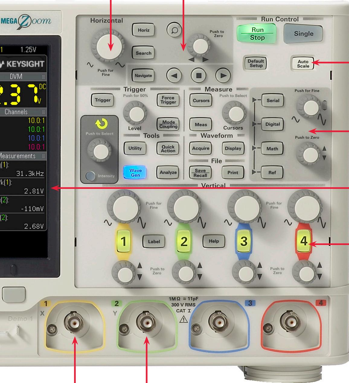
Autoscale lets you quickly display any analog or digital active signals, automatically setting the vertical, horizontal and trigger controls for the best display, while optimizing memory
