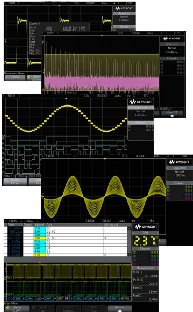
After capturing a serial bus communication, you can easily perform a search-and-navigation operation based on specific criteria of your interest. Note, the digital channels and serial protocol analysis cannot be used simultaneously.
