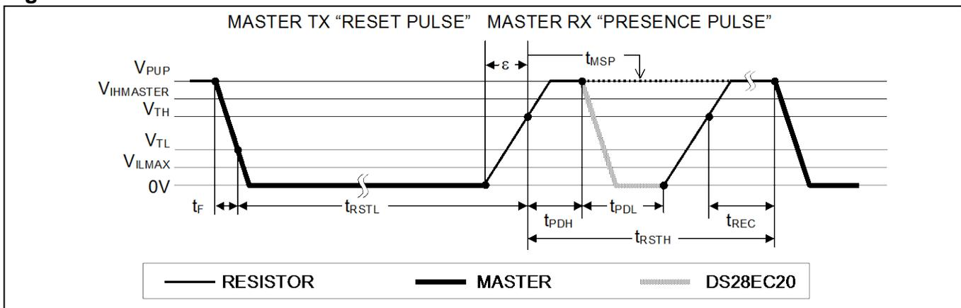
After the bus master has released the line it goes into Receive mode. Now the 1-Wire bus is pulled to  $V_{PUP}$  through the pullup resistor, or in case of a DS2482-x00 or DS2480B driver, by active circuitry. When the threshold  $V_{TH}$  is crossed, the DS28EC20 waits for  $t_{PDH}$  and then transmits a presence pulse by pulling the line low for  $t_{PDL}$ . To detect a presence pulse, the master must test the logical state of the 1-Wire line at  $t_{MSP}$ .
