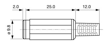
Cable diameter max. 4.0 mm
