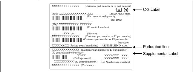
Label II-A: Label on Outer box [D Label] (100mm × 100mm)
