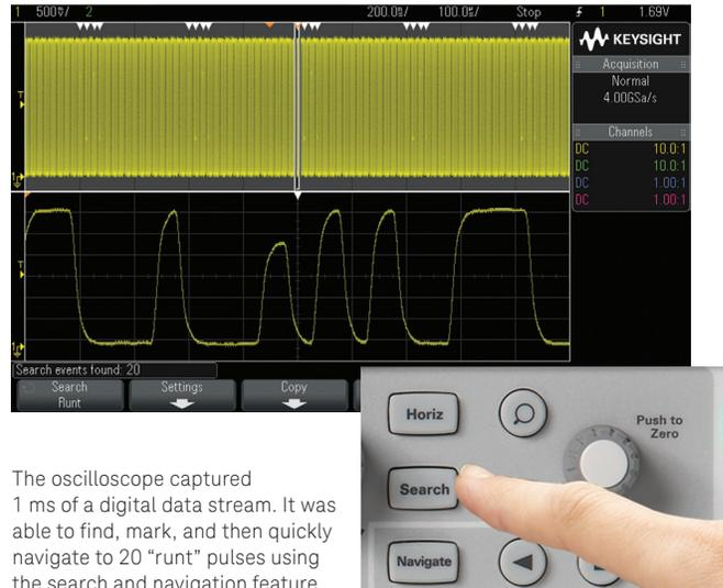
The oscilloscope captured 1 ms of a digital data stream. It was able to find, mark, and then quickly navigate to 20 "runt" pulses using the search and navigation feature
