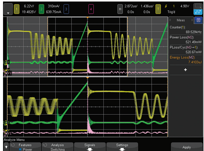
Figure 1. By measuring the switching loss and conduction loss, you can characterize the instantaneous power dissipation in a switching power supply.
