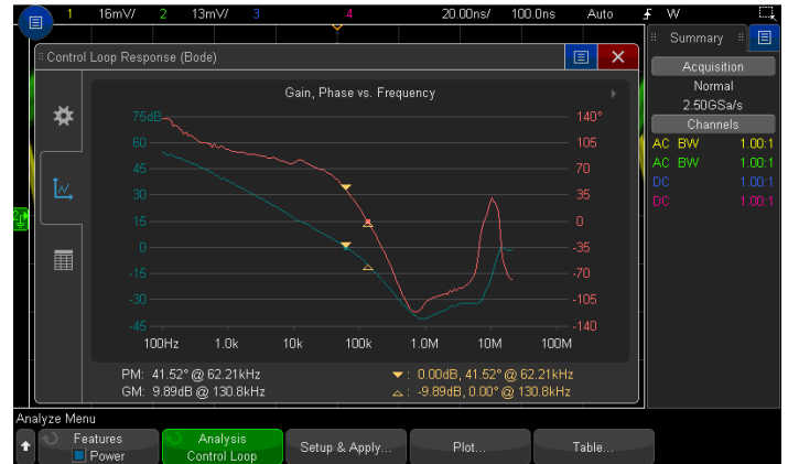
Figure 13. Control Loop Response gain measurement using an InfiniiVision X-Series oscilloscope.
