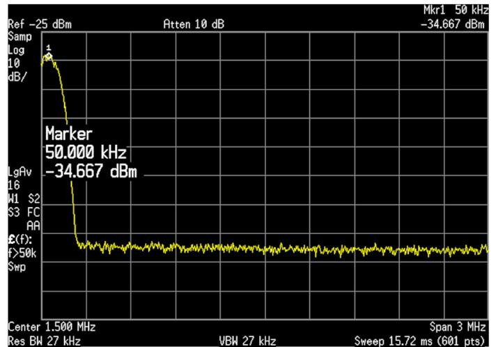
The images show approximately 10 dB increase in amplitude at 50 kHz when the bandwidth is reduced 10x. You can see how the signal energy is increased in the frequencies of interest when the bandwidth is reduced, instead of being spread over a very wide bandwidth with lower amplitude at all frequencies.
