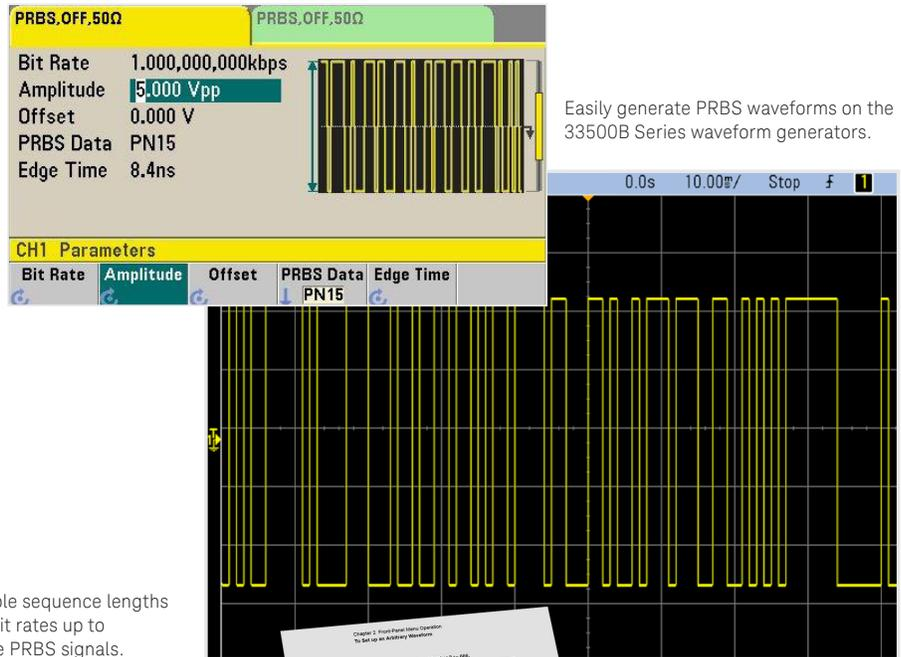
You can select multiple sequence lengths (such as PN15) and bit rates up to 50 Mbit/sec to create PRBS signals.
