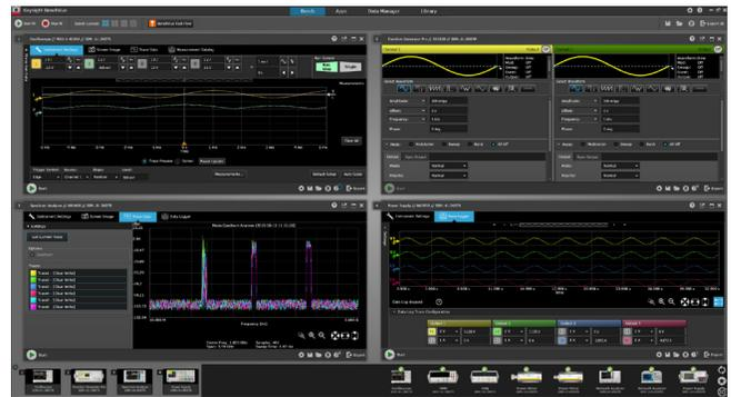
See your measurements across instruments in one place to quickly correlate measurement activities and obtain actionable insights. Control your waveform generator to set waveform properties and load custom arbitrary waveform from files or drag-and-drop from an oscilloscope.
