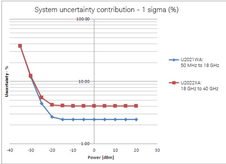
Note: The above graph is valid for conditions of free-run operation, with a signal within the video bandwidth setting on the system. Humidity < 70 %.
