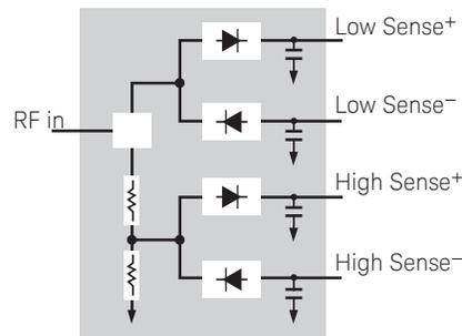
This technique ensures diodes in the selected signal path are kept in their square law region—with output current and voltage proportional to input power. The diode pair/attenuator/
