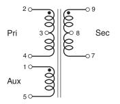
Note: By using stamps as the primary and primary boards as the secondary, a step-up transformer, up to 1:12 turns ratio, can be created.
