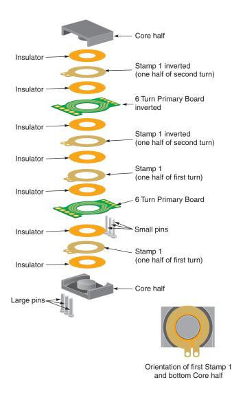
Figure 5. Exploded view of the Sample Transformer
