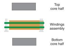
Figure 1. Major Components of a Planar Transformer
