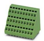
PCB terminal block, nominal current: 12 A, nom. voltage: 400 V, pitch: 5.08 mm, number of positions: 1, connection method: Spring-cage connection, mounting: Wave soldering, conductor/PCB connection direction: 45 °, color: green. Single module for the custom grouping of different numbers of positions. An end terminal block is also needed to terminate the block (see accessories). Blocked items with different numbers of positions are also available.
