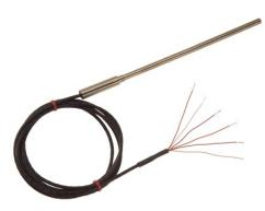
Mineral Insulated Duplex PRT's with two independent PT100 detectors inside tip of probe. This allows one probe to be connected to two measurement or control devices; alternatively, one sensor may be used as a primary and the other as a backup, eliminating the need to remove and replace the probe if one of the sensors should fail.
