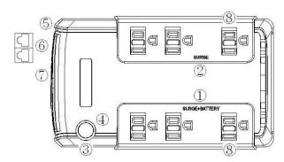
The unit has three battery powered/surge suppression outlets to ensure temporary uninterrupted operation of your equipment during a power failure. (DO NOT plug a laser printer, paper shredder, copier, space heater, vacuum, sump pump or other large electrical device into the "Battery and Surge Protected Outlets." The power demands of these devices will overload and possibly damage the unit.)
