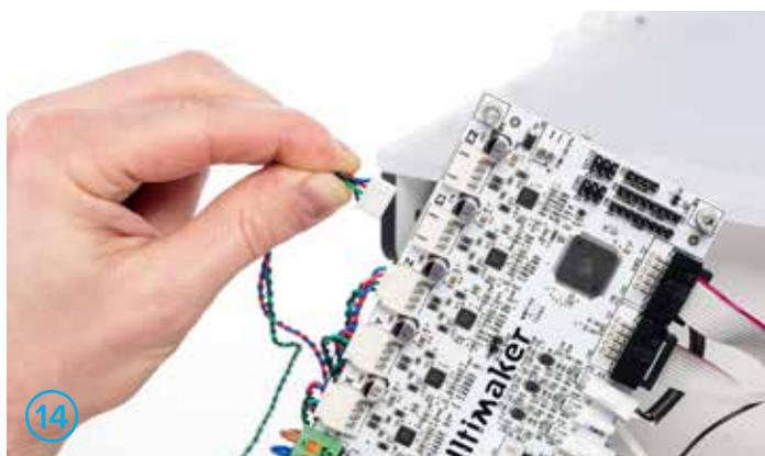
12. There's a ferrite core around the motor cables. Open it so you can remove the feeder motor wire completely. (It's possible that your Ultimaker is older and doesn't have the ferrite core). Fig. 15.
