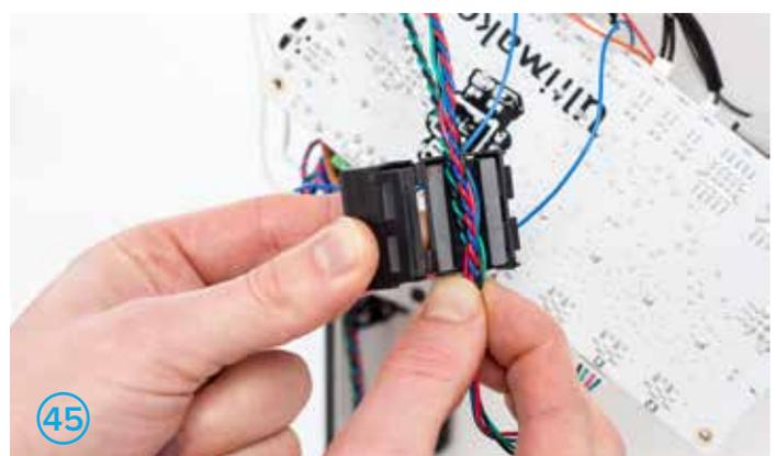
8. Connect the wires of the heater cartridge to the green terminal HEATER 1. Press at the top of the terminal with the flat screwdriver and insert the wires. Fig. 46.
