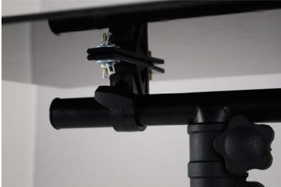
6. Tighten the screws from above using a screwdriver to secure everything into place.
