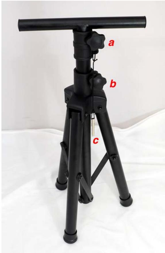
Note that knob (a) is for raising and lowering the T-bar, knob (b) is for opening and closing the tripod legs, and bar (c) secures the t-bar in place.
